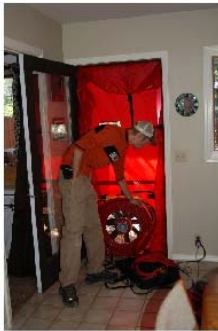
Auditor preparing for blower door test to determine house tightness.
