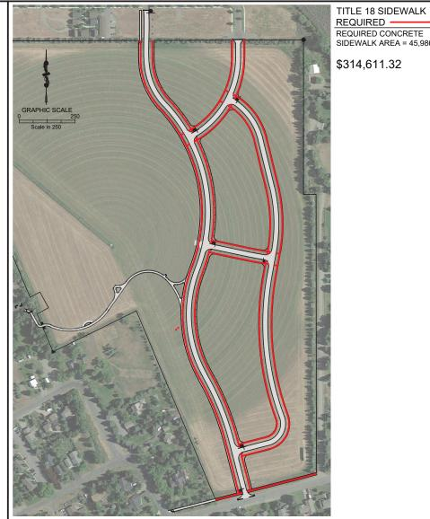
REQUIRED -REQUIRED CONCRETE SIDEWALK AREA = 45,986 SF
