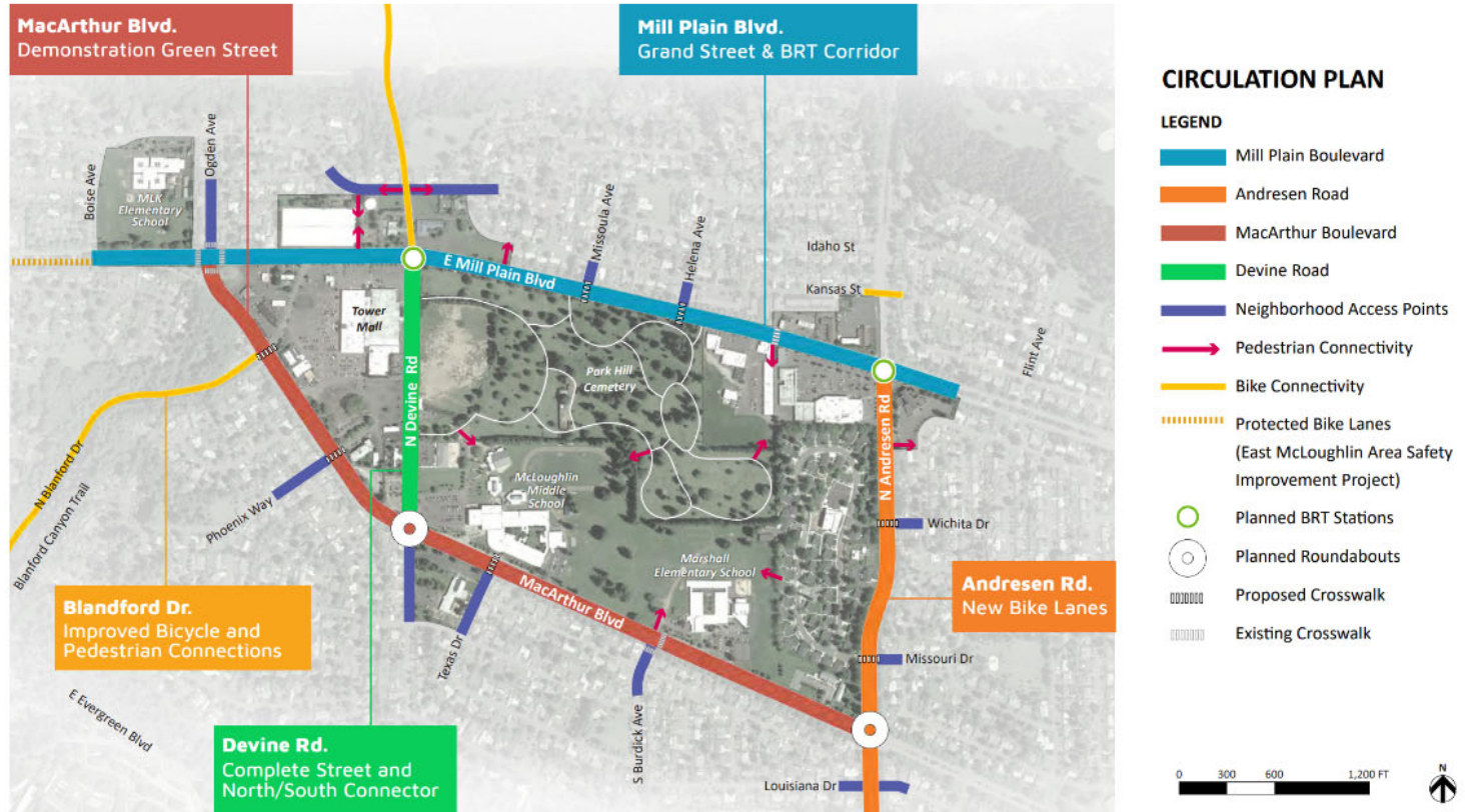
Fig 20: Proposed Access and Circulation Improvements
