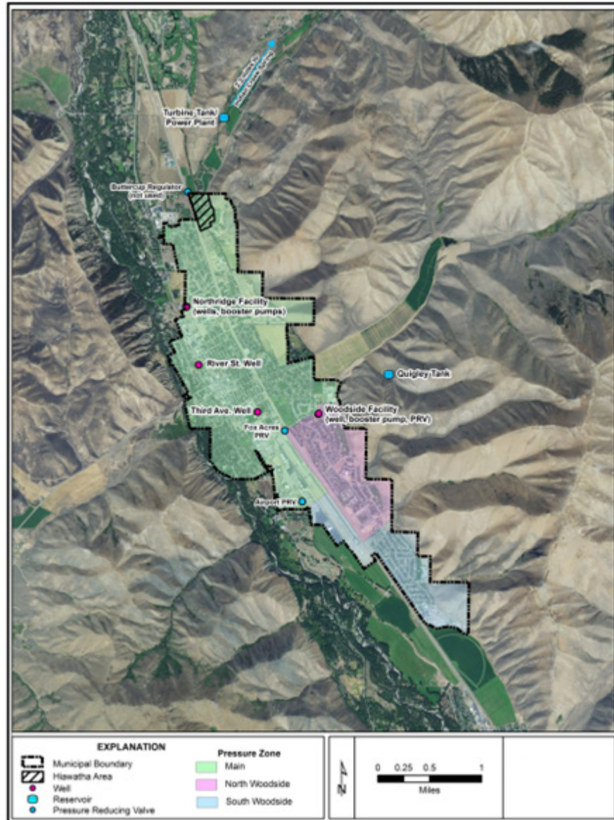
Figure 13: City of Hailey Existing Water System Facilities
